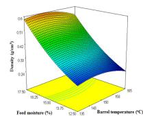
Figure 1. Effect of barrel temperature and feed moisture content on product density.
