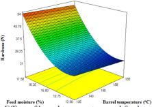
Figure 3. Effect of barrel temperature and feed moisture content on product hardness.
